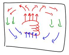
Convection speeds up the process of heat transfer from the hot object to the surroundings.
