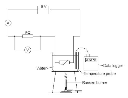
To calibrate the thermistor to measure temperature, the student placed the thermistor in a beaker of water at 0 °C and took the voltmeter reading. The student then heated the water slowly with a Bunsen burner. The student recorded the reading on the voltmeter every 10 °C.
