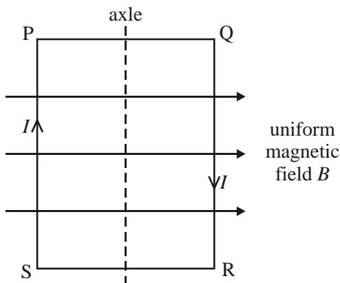
A coil, mounted on an axle, has its plane parallel to the flux lines of a uniform magnetic field  $B$ , as shown. When a current  $I$  is switched on, and before the coil is allowed to move,
